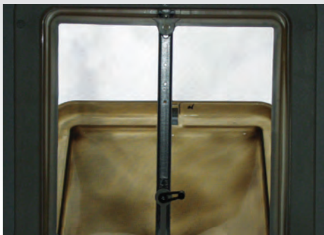
PASSIVE ROOF VENT - These vents can be configured to draw air into the trailer and include crank handles and screens. Powered vents are also available.
