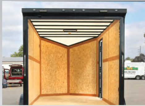
TRANSLUCENT ROOFING - An easy solution to light inside of the trailer during the working day—a common option for enclosed construction and landscape trailers.
