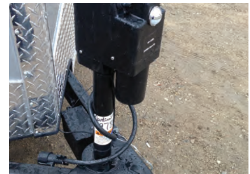
12-VOLT POWERED TONGUE JACK - This power jack makes hooking up to heavy-trailers as easy as the push of a button.
