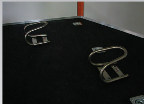
MOTORCYCLE WHEEL CHOCKS - Wheel chocks are easily removable—opt for the flush-mounted in-floor steel models.
