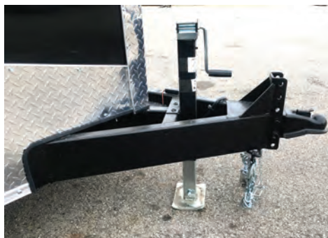
HEAVY DUTY JACK - This fixed-mount heavy duty jack is installed to take the maximum load on its oversized foot.
