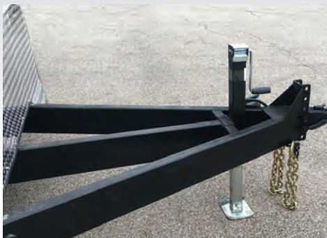
EXTENDED TUBE TONGUE - Tongue extensions are available to accommodate specialty tow vehicles.
