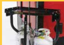
Tongue mounted LP tanks w/ optional generator stand
